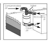
1. Air may be recirculated and continuously cleaned within the shelter.
